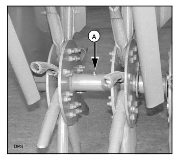
Figure 4 . Lubrication Points
